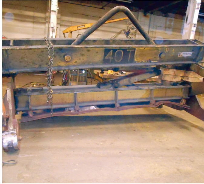
40-ton slab tongs before remanufacturing
