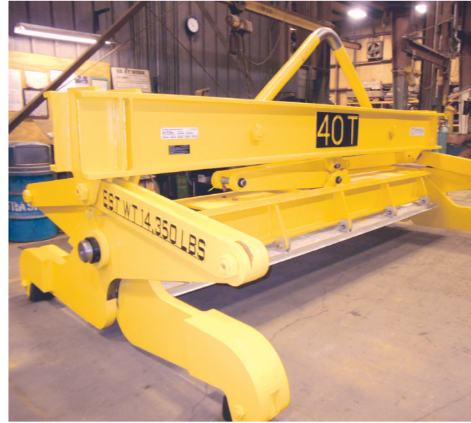
40-ton slab tongs after remanufacturing
