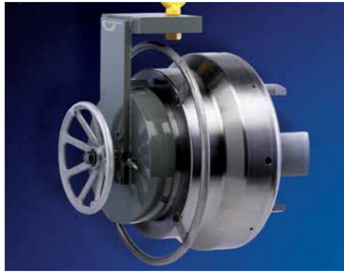
Removable Mount mounting tool
