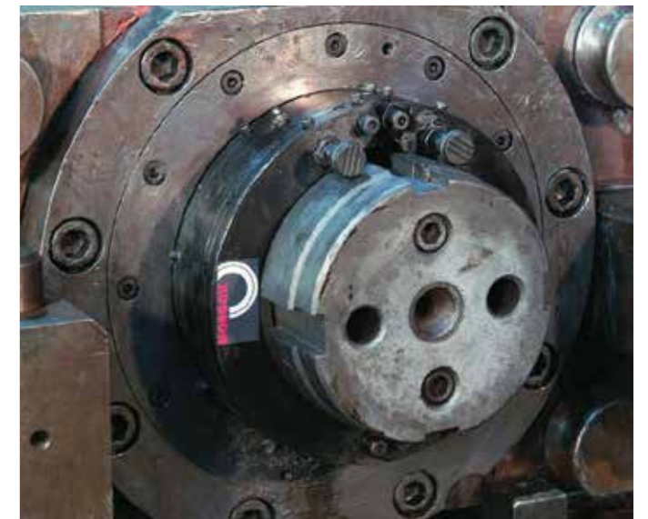
MORGOIL LD™ lock on work-up roll
