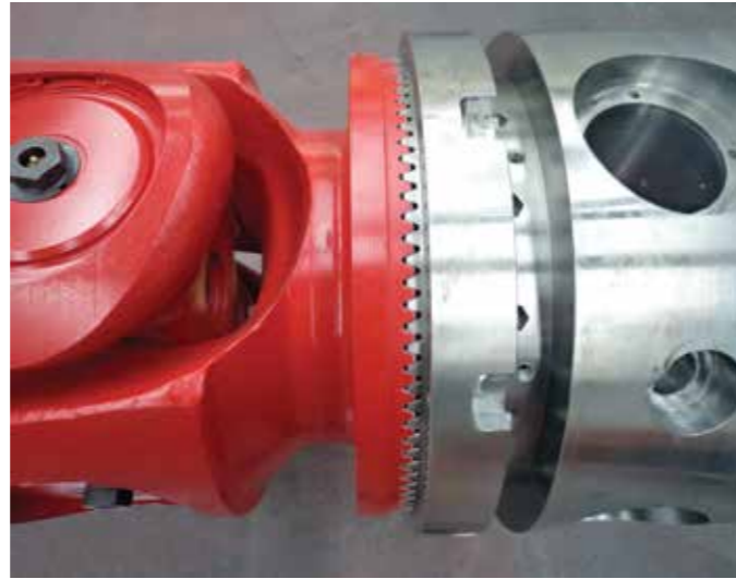
Universal drive system featuring Hirth coupling
