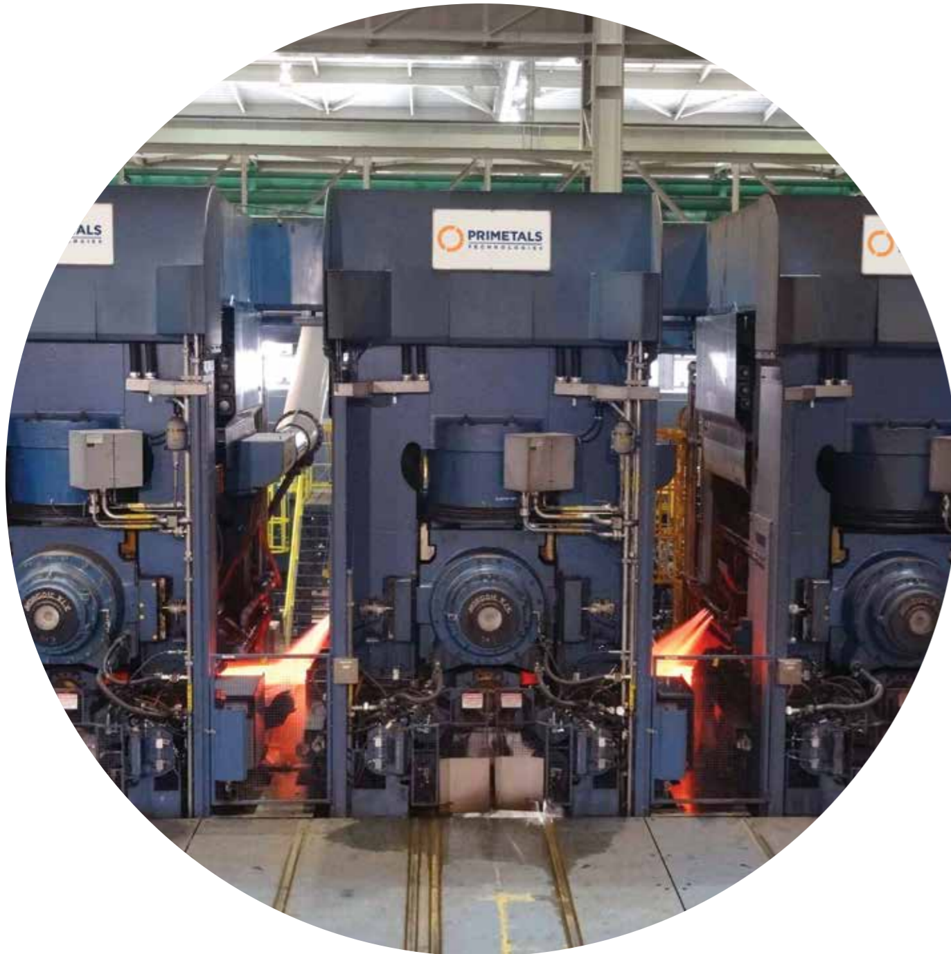
MORGOIL® Bearing equipped finishing stand at Allegheny Technologies Incorporated's new hot rolling plant located in Brackenridge, PA, USA. These 58-86 MORGOIL KLX® Bearings are the highest load capacity backup roll bearings employed on a hot strip mill.
