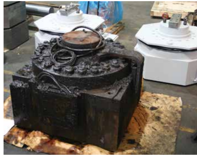
HAGC Cylinders before and after reconditioning
