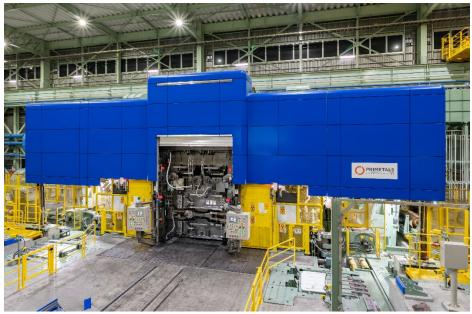
Nippon Yakin Kogyo's new split-housing HZ-Mill from Primetals Technologies replaces two monoblock cold rolling mills.
