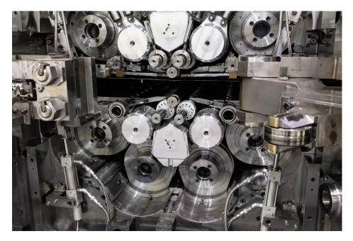
The new reversing cold mill produces coils with thicknesses down to 0.2 millimeters at rolling speeds up to 1,000 meters per minute.
