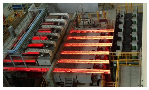
Primetals Technologies will supply and implement a 6-strand bloom casting machine for high-quality production demands.
