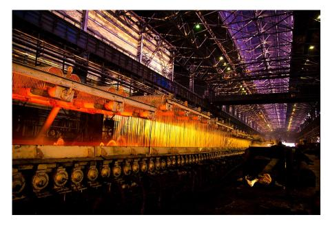
Cooling section at SAIL Bokaro's hot-strip mill. Primetals Technologies' modernization encompassed automation equipment for the finishing mill, cooling section, down coiler, and coil conveyor.
