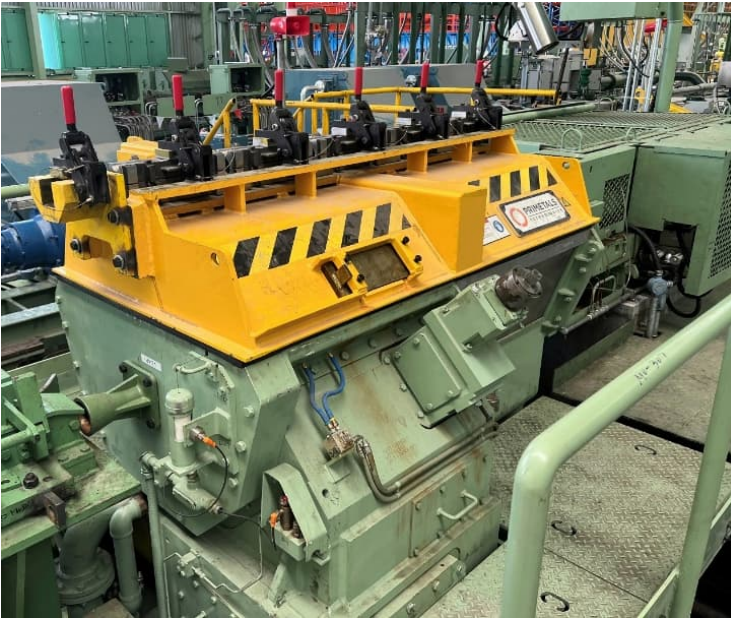
One of the newest solutions from Primetals Technologies – the eDrive mini-finishing mill.
