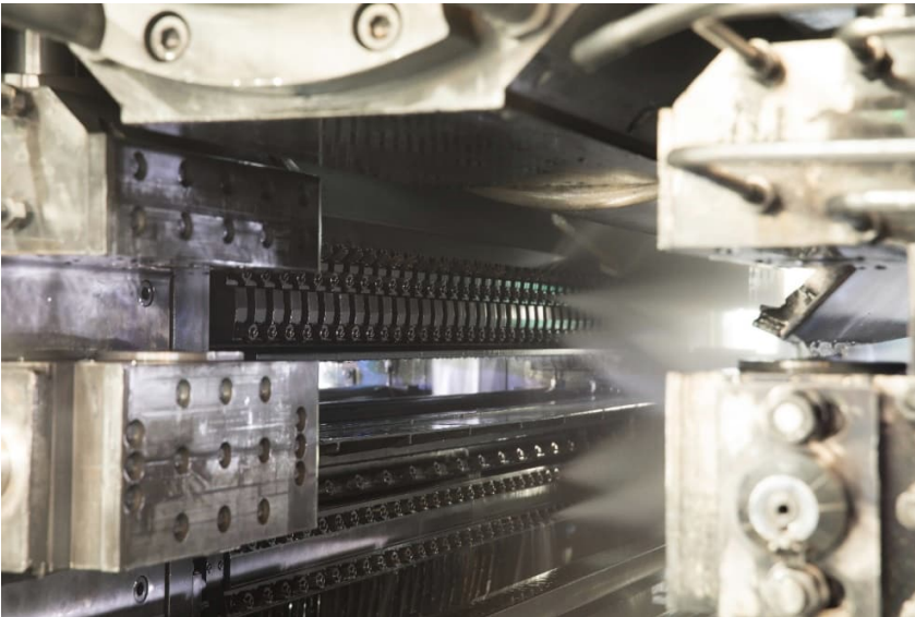
ISV Spray System from Primetals Technologies installed on an aluminium foil mill.
