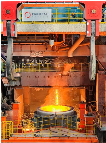
Picture of the first heat at Huaigang's EAF Quantum supplied by Primetals Technologies.
