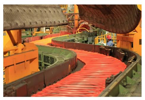
Curved section of Primetals Technologies' Stelmor Conveyor for future in-line direct solution treatment (DST) processing.
