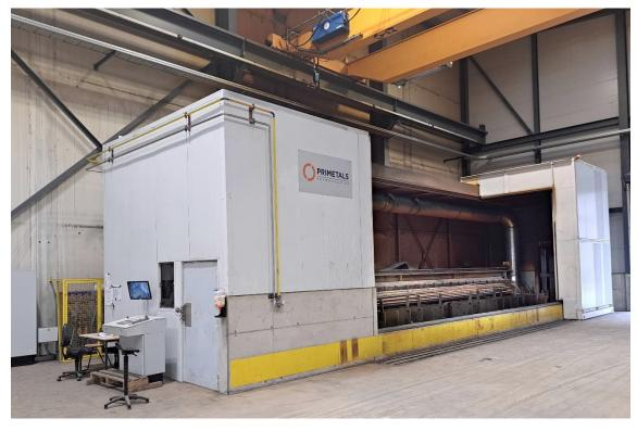
Primetals Technologies' scrap torch-cutting machine results in heavily reduced noise levels and a streamlined process for the sorting and managing of scrap.
