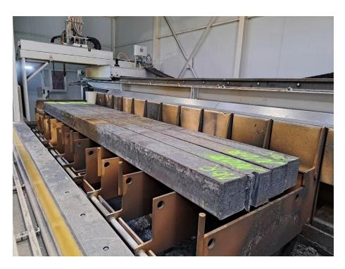
The scrap torch-cutting machine from Primetals Technologies handles various types of scrap including billets, bundles of rolled bar, ladles, and tundish scull.
