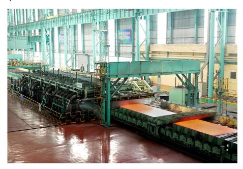
MULPIC - world-leading plate cooling technology from Primetals Technologies.
