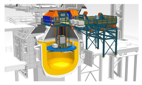
Primetals Technologies is responsible for engineering, supply, manufacturing, startup, and advisory service for construction of the new relining machine.
