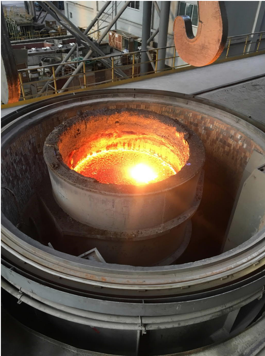
Vacuum degassing plant (VD) from Primetals Technologies
