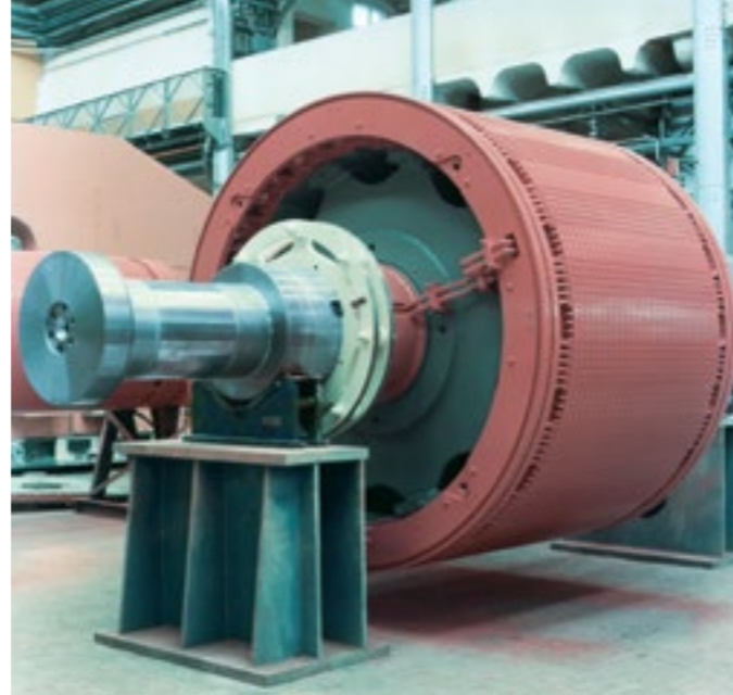
Maintenance-free cylindrical rotor
