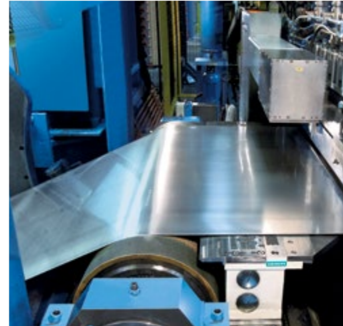
Non-contact - flatness measurement and control
