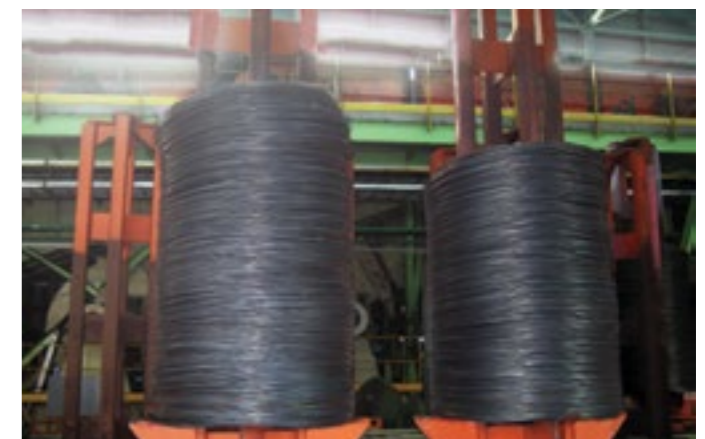
Example of coil height reduction possible with new SR Series pipes, producing the coil on the right, compared to standard pipe on the left
