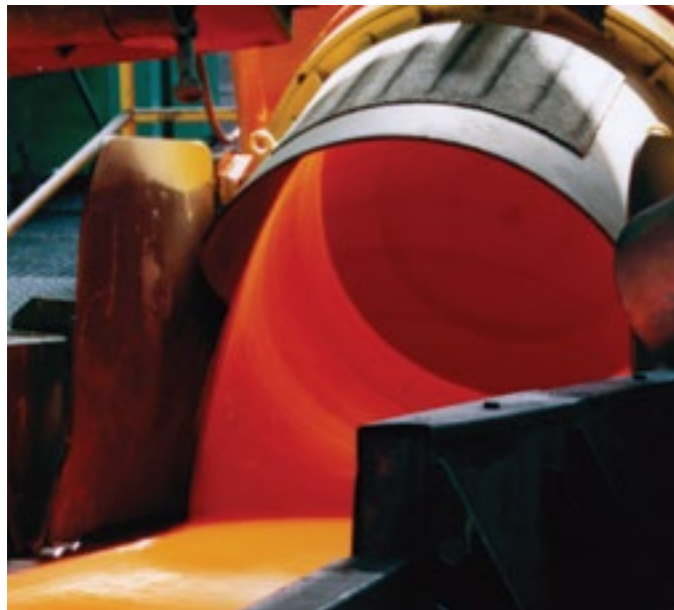
Morgan High Speed Laying Head for consistent high speed operation
