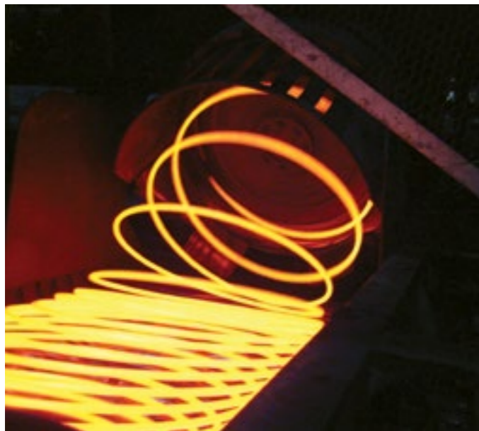
Mechatronics control for consistent rings throughout the coil
