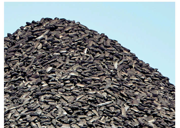
Hot briquetted iron
