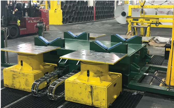
Work roll chocking station
