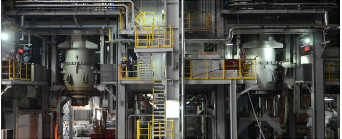
Highly productive on a small footprint - RH plants with CVL Lifting system
