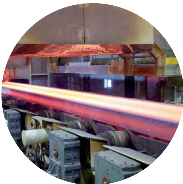
Single stainless slab caster, Outokumpu, Tornio, Finland
