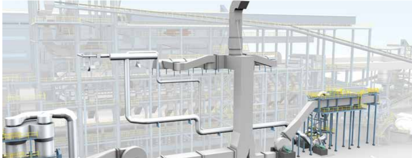
Selective Waste Gas Recirculation System
