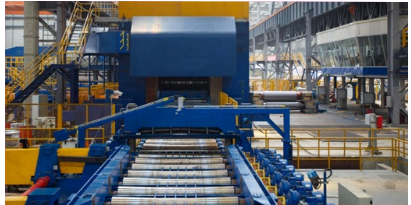
Hot Finishing Mill Entry Side
