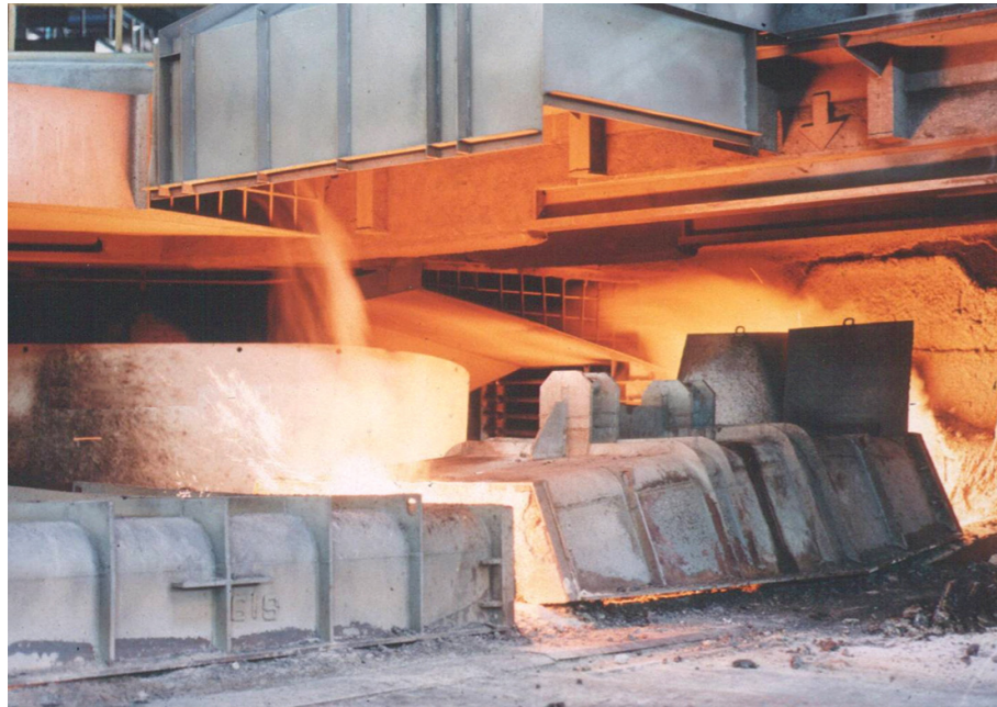
Casthouse taphole extraction
