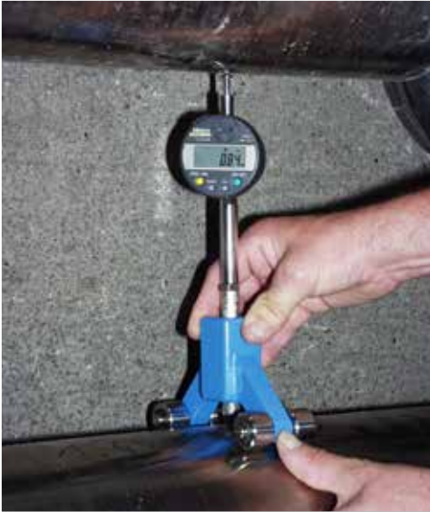
Roll gap measurement with GapChecker
