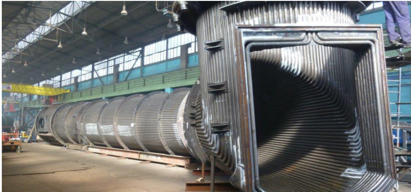
Partially assembled cooling stack in the workshop
