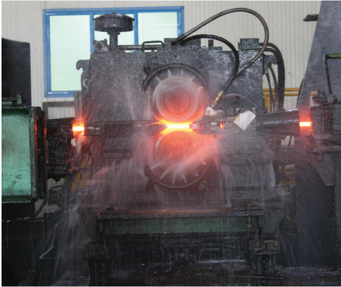
Powered slitter in a high speed bar mill
