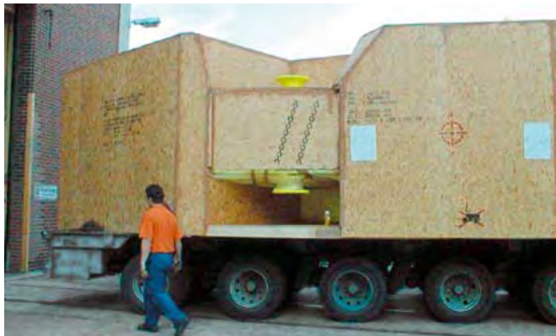
Example: add-on packaging with OSB-cladding and marking to prohibit the use of forklift trucks as well as marking of the centre of gravity
