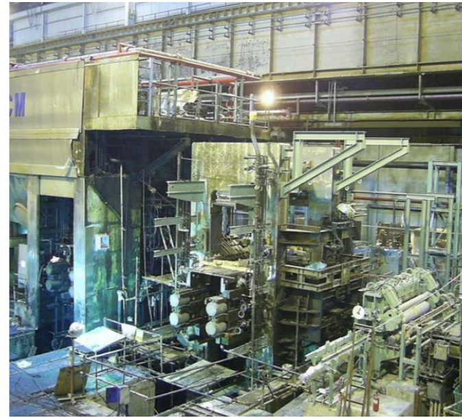
Additional no. 0 stand mill installation at no. 1 PLTCM at Kwangyang, POSCO, South Korea
