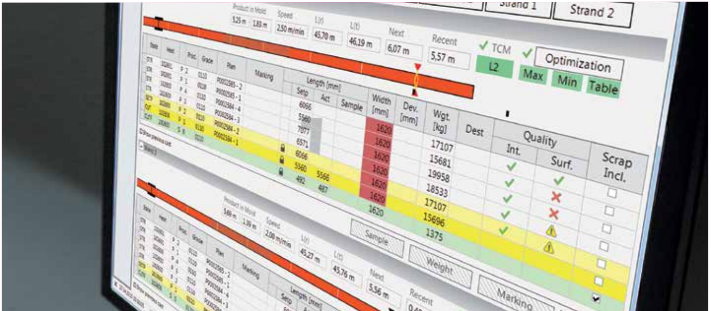
Cutting overview screen of a two-strand slab caster
