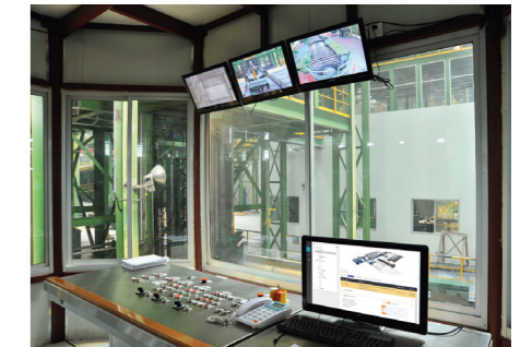
The ALEX installation at a hot strip mill in Mexico warned the maintenance department of an inaccuracy in the roll force measurement, recommended to calibrate the measurement system and prevented a production loss of seven hours.
