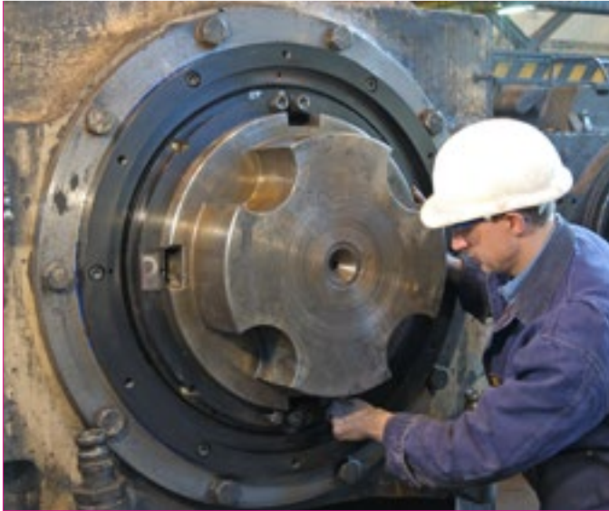
Morgoil® LD Locking system upgrade
